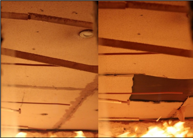
Photo 17: The exposed face of sample (After test duration of 10 & 20 minutes)
