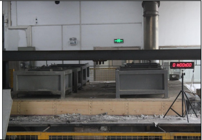
Photo 22: The unexposed face of sample (After test duration of 60 minutes)
