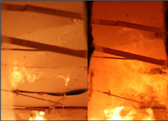
Photo 21: The exposed face of sample (After test duration of 50 & 60 minutes)
